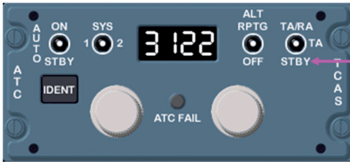
Fig 3: Basic ATC/TCAS control panel
