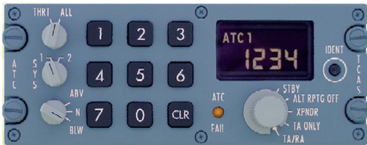
Fig 2: Gables 40 ATC/TCAS control panel
